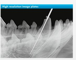
When conventional image plates are used for non-dental radiography, the laser beam diameter is focused to 50  $\mu m$ (10 lp/mm), which guarantees brilliant low-noise images with high contrast for best diagnosis.
